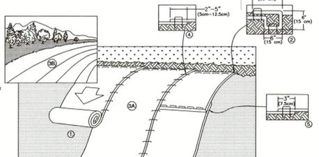
1. PREPARE SOIL BEFORE INSTALLING ROLLED EROSION CONTROL PRODUCTS (RECP's), INCLUDING ANY NECESSARY APPLICATION OF LIME, FERTILIZER, AND SEED.
